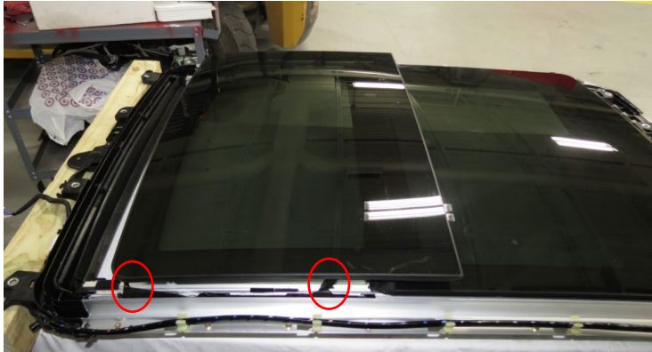
Figure 7. Aisin outer slider sunroof – front slides outside of rear panel.
