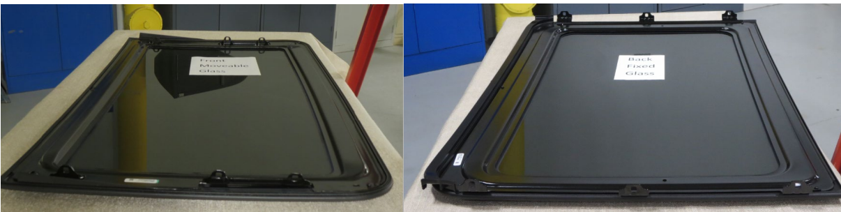
Figure 3. F-150 sunroof panels – left: front moveable panel, right: rear fixed panel.
