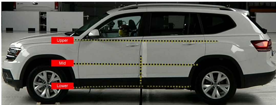
Figure 4. Measurement locations for external crush
