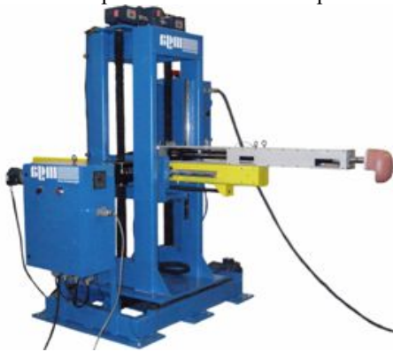
Figure 10. Ejection guided impactor with 18 kg featureless headform.
