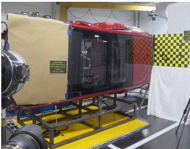
Figure 6. Sunroof panel glued to roof of vehicle with polyurethane.
