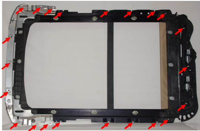
Figure 2. Red arrows indicate where sunroof module was bolted to the roof of the vehicle.
