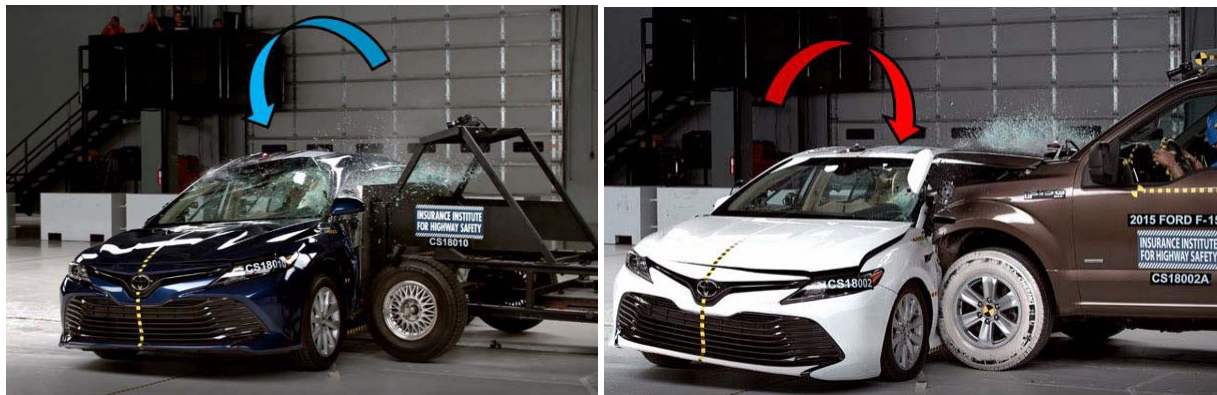
Figure 6. Vehicle dynamics comparison between Toyota Camry struck by the MDB (left) and Ford F-150 (right) at 60 km/h during maximum roll
